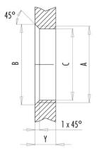
Installation direction: o-ring sits on chamfer.
